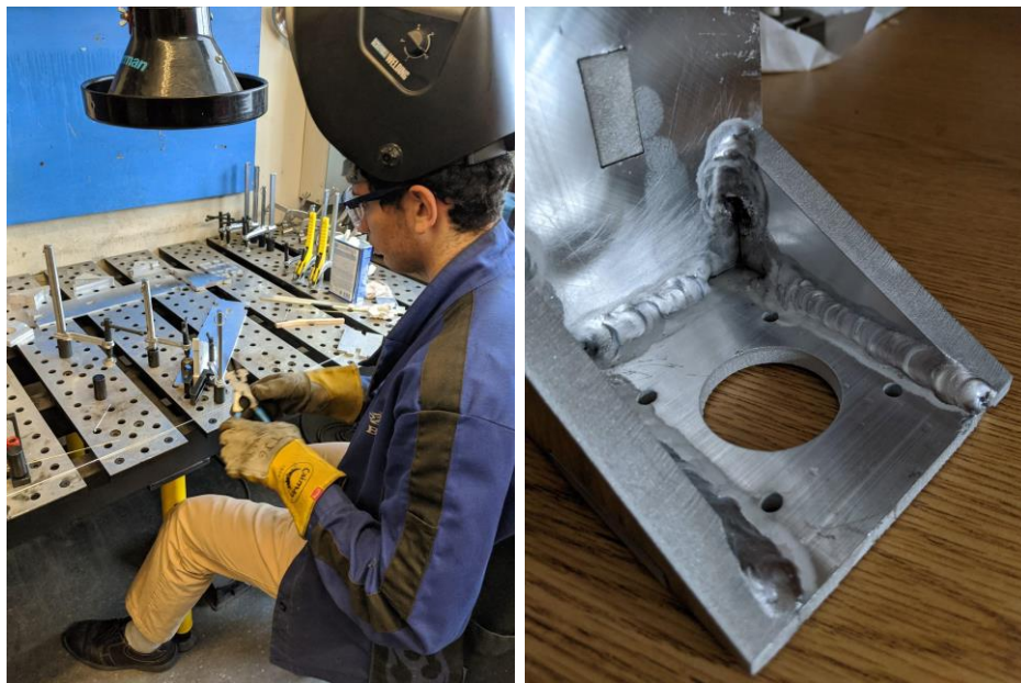
Figure 5-3: Jigging and welding the aluminum plates for the CNC foam cutter railings.
