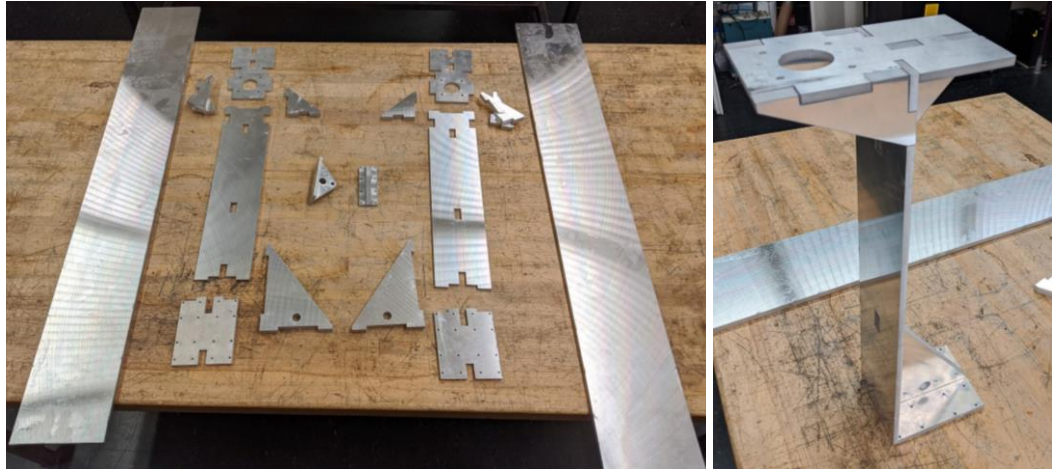
Figure 5-2: Water-jet aluminum pieces for the foam cutter railing. On the right is shown how these pieces are to be jugged together for ease and accuracy of welding.
