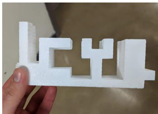
Figure 5-9: "IcyQ" letters cut out of EPP foam using the 4-axis CNC foam cutter.
