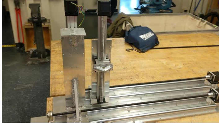
Figure 5-4: Both sides of the 4-axis CNC foam cutter with mechanical fabrication and assembly fully complete.
