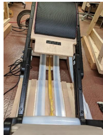
Figure 5. Yellow hoist strap attached to foot panel shaft.
